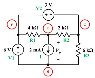
The incomplete text file shown below is intended to describe this circuit so that it can be analyzed with PSpice to determine the value of  $V_x$ . Fill in the missing parts.
